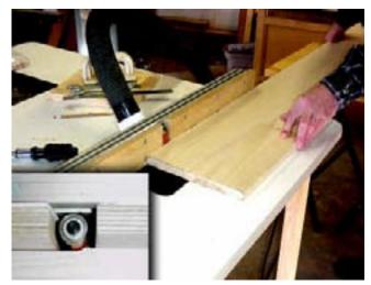
When I am joining boards, I first place them together and mark the boards with a light "arc" witness mark. Then, I run one board with the mark down and the other one with the mark facing up. This way, if the router is not exactly 90o, the joint will still be perfect. I do this when using the jointer as well.
