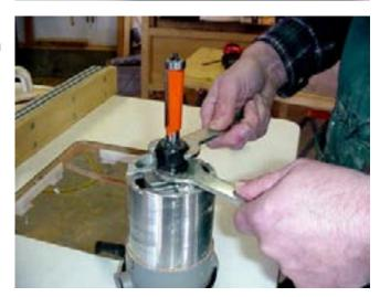
Then, install the router and adjust the fence so that the left-side of fence is in exact alignment with the straight bit bearing. The gap between the straight edge and the right fence should equal the Formica shim thickness. Be sure to move the two fences as close as possible to the bit—as a matter of practice, I leave about 1/8" space around the bit.
